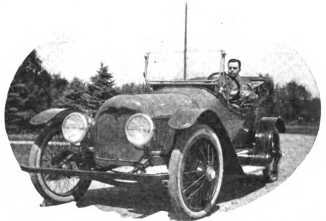
One of the new Beardsley electric roadsters manufactured in Los Angeles, Cal., which is claimed to do better than 30 m.p.h. and to be good for 85 to 100 miles per charge
